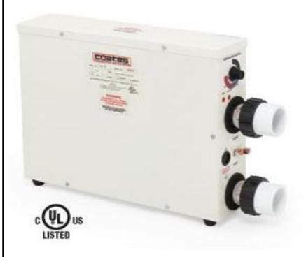
The built-in pressure switch prevents operation when there is no water flow and allows operation at flow rates between 15GPM and 80GPM. The stainless steel tank is designed to optimize heat transfer by directing the water flow over the incoloy elements efficiently.
